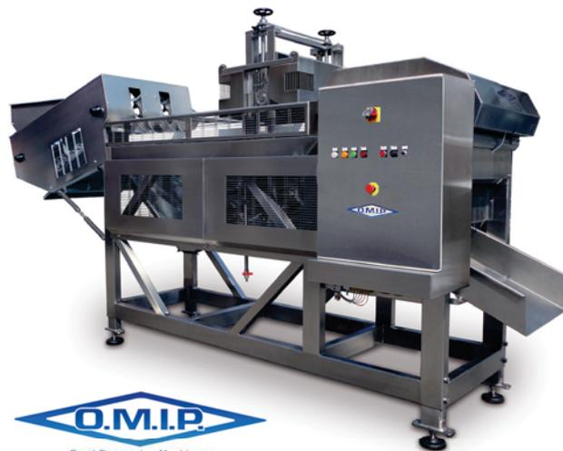
The **KR8 Peach Repitter Machine** enables to re-pit peaches with stone problems. It re-pits 320 half peaches per minute with any degree of ripeness and any variety (clingstone, freestone and nectarine) allowing to eliminate labour for this operation. The machine has been designed to make cleaning and maintenance operations easier.
